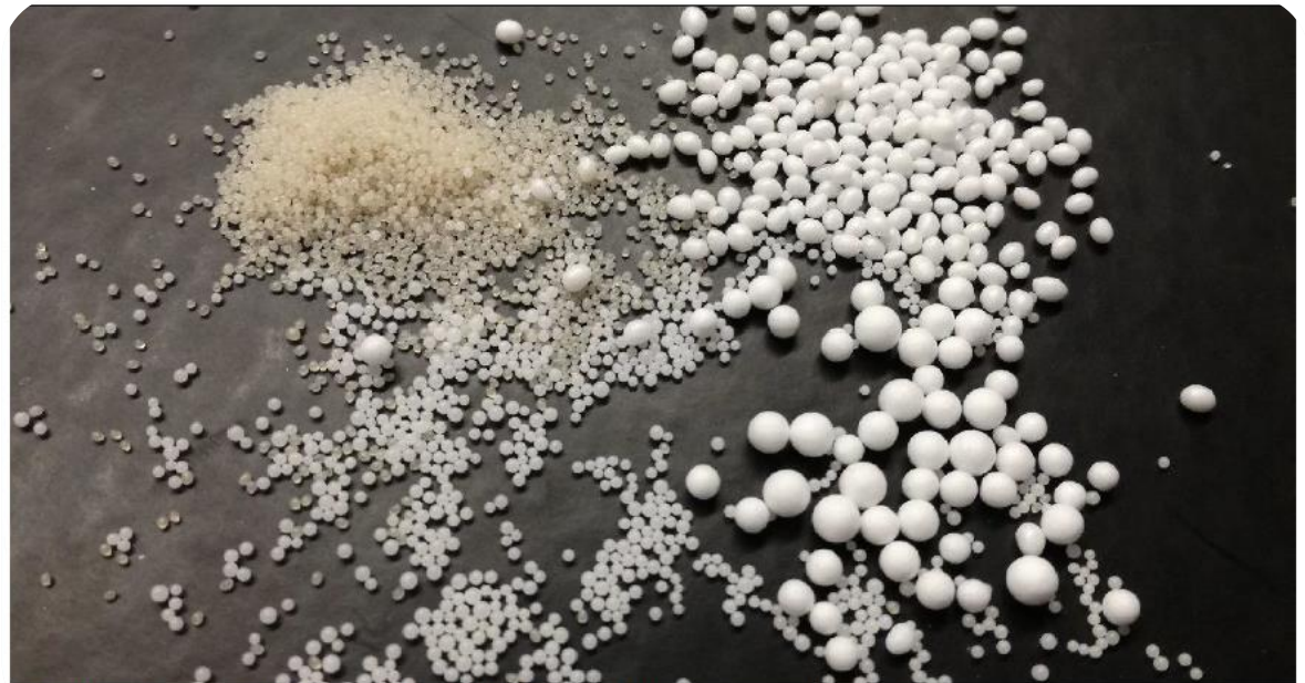
Bild 2: RE710e from BEWI in comparison with a standard EPS raw material
